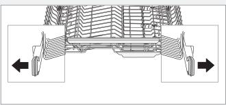
Pull out the top cutlery tray. Press the top spray arm up and unscrew the spray arm bearings counterclockwise to remove the spray arm.
